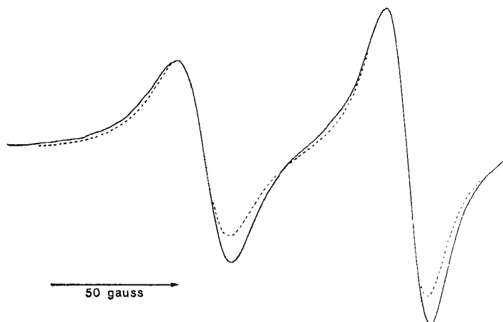
Figure 7. The first two hyperfine lines in the spectrum of vanadyl acetylacetonate dissolved in the nematic mesophase of 4,4'-dimethoxyazoxybenzene. The dotted lines show a reconstruction based on a symmetric Lorentzian line shape.
